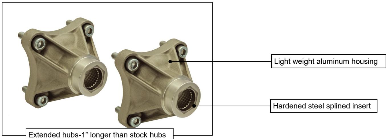
Extended hubs will lengthen your tread width by 1" on each side. These hubs can be used instead of using wheel spacers.
