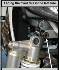
The upper shock mount bolt as been removed.
