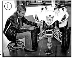
Note: The technician carefully removes the nut and bolt from the shock.
