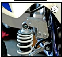
2) Remove the top bolt that holds the shock in place. Place the main block where the shock was. Due to chassis Variations, you may need to enlarge the main block hole to use the stock bolt. **Note:** Lowering kit plates are a left right orientation!
