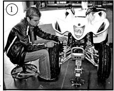
Note: The technician carefully removes the nut and bolt from the shock.
