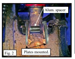
3) The 2 plates of the lowering kit go on the outside of the old shock mount. Put the bolt through the plates and brackets. The aluminum spacer goes between the shock mounts. In some cases you may need to trim the plates to get the holes to line up.(See fig. 2)
