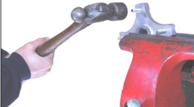
THE WRONG WAY TO REMOVE STUDS
