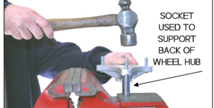
THE RIGHT WAY TO REMOVE STUDS
