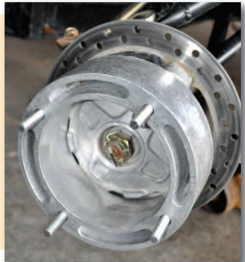
With the wheel spacers installed the brake is no longer tucked inside the wheel, but unless you do a lot of riding in the rocks it won't matter. Expect a slightly bigger turning radius though.
