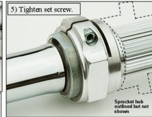
6) This is how the Posi\*Lock looks installed. Note that the inner sleeve covers the top of the snap ring. If the Posi\*Lock is installed backwards the c-clip will be pushed out of the groove by the flat side of the main nut. The inner sleeve always faces the wheel hub.
